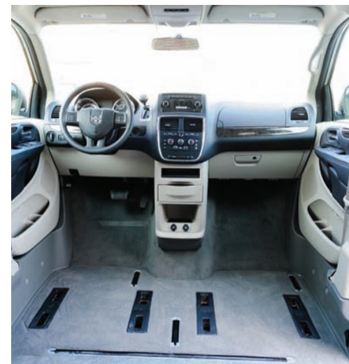
▲ Amerivan's front seats can be easily removed and replaced, with a locking mechanism operated by a quick-release foot pedal.
