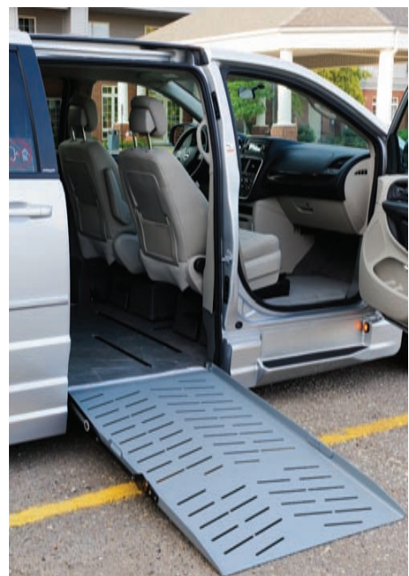
▲ Amerivan is equipped with an automatic load leveling suspension. This feature will allow the van to kneel making entering and exiting convenient.
